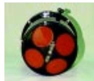
Transducer and electronics: 6061 aluminum transducer head with four beams at 30 degrees from vertical in convex configuration, electronics assemblies, fluxgate compass, pitch, roll and temperature sensor.
