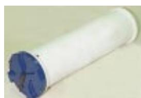
Pressure case: 1500m depth rated 6061 aluminum pressure case. End cap with wet-mateable connector and dummy plug.
