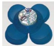
Transducer and electronics: aluminum transducer head with four beams at 20° from vertical in a convex configuration, temperature sensor, electronics assemblies, fluxgate compass, pitch and roll sensors.
